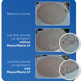
The Low Fines Concrete without MasterMatrix LF bleeds at the border, a symptom of instability: upon the introduction of MasterMatrix LF no water is released, and the overall concrete aspect is very homogeneous and stable, comparable to the reference concrete, despite the reduced amount of fines.
