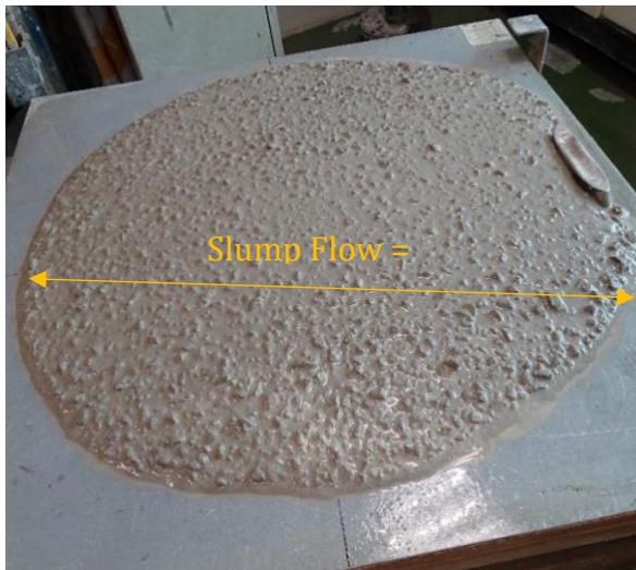
Low Fines Concrete without MasterMatrix LF
