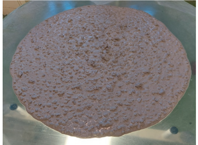
Fig. 7: On the left reference mix (400 kg/m 3 of CEM I 52,5 R), on the right low clinker mix (370 kg/m 3 of CEM II/A-LL 52,5 R)
