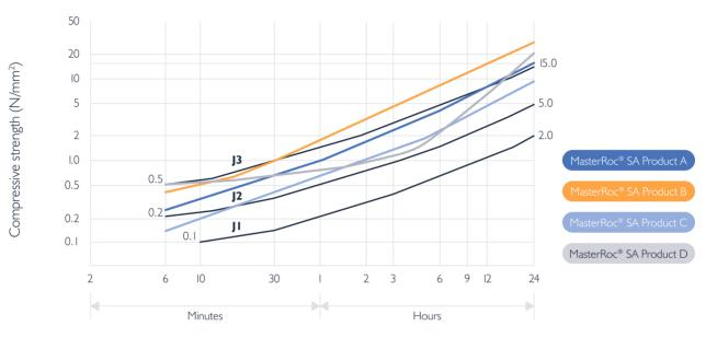
Recorded compressive strength developments by selected alkali-free set accelerators in comparison with JI, J2 and J3 standard requirements based on the Austrian Guideline for sprayed concrete.
