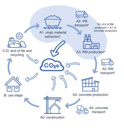
1 Typical cradle to gate GWP for concrete, based on Master Builder Solution case studies, calculated with OneClick LCA
