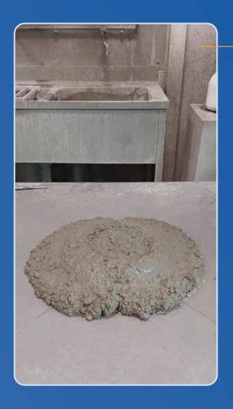
Reference concrete mix (conventional superplasticizer): CEM II/A-LL 42.5, 307 kg/m³
